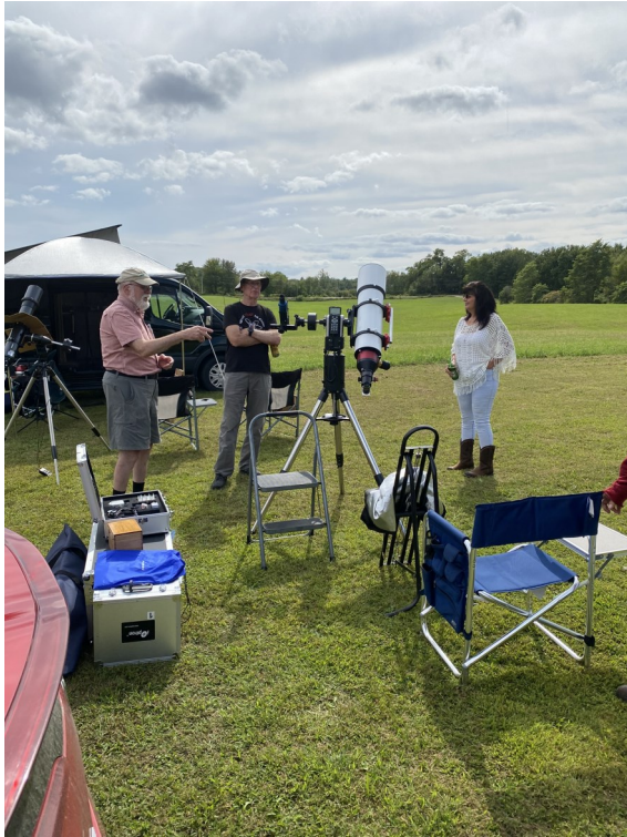
Dwight's Lunt 152mm H \alpha telescope set-up. Solar viewing on one side of the mount. And looking through Dwight's spectrometer on the other side of the mount.
