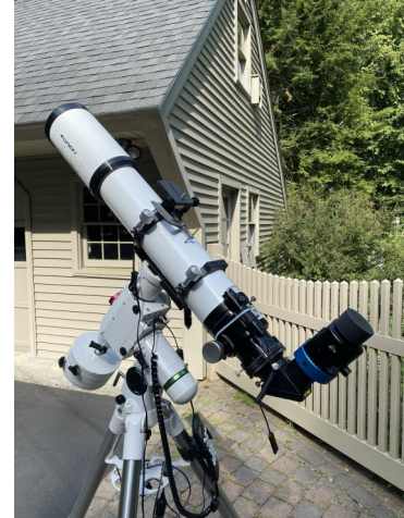
Orion EON 115mm (4.5") ED Triplet Apo Refractor; f/7 Focal Length: 805mm.
