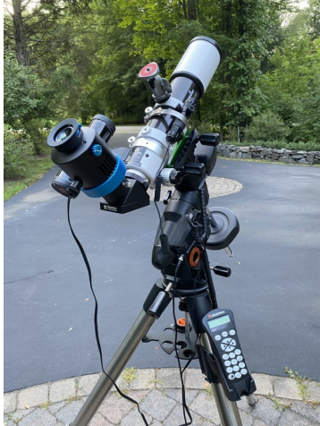
Skywatcher Evostar 72 ED (2.8") Apo Refractor; f/5.8 Focal Length: 420mm.
