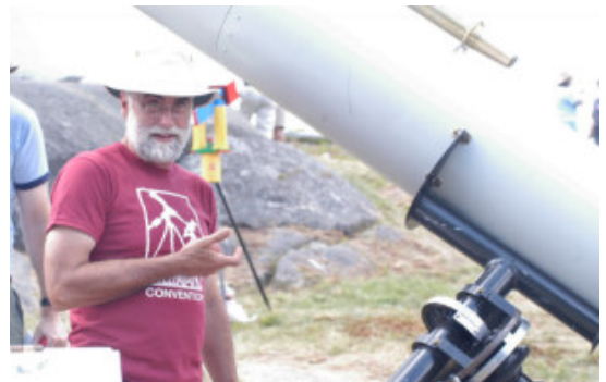
Jan standing next to the 12.3" f/10 Newtonian on a German Equatorial Mount
